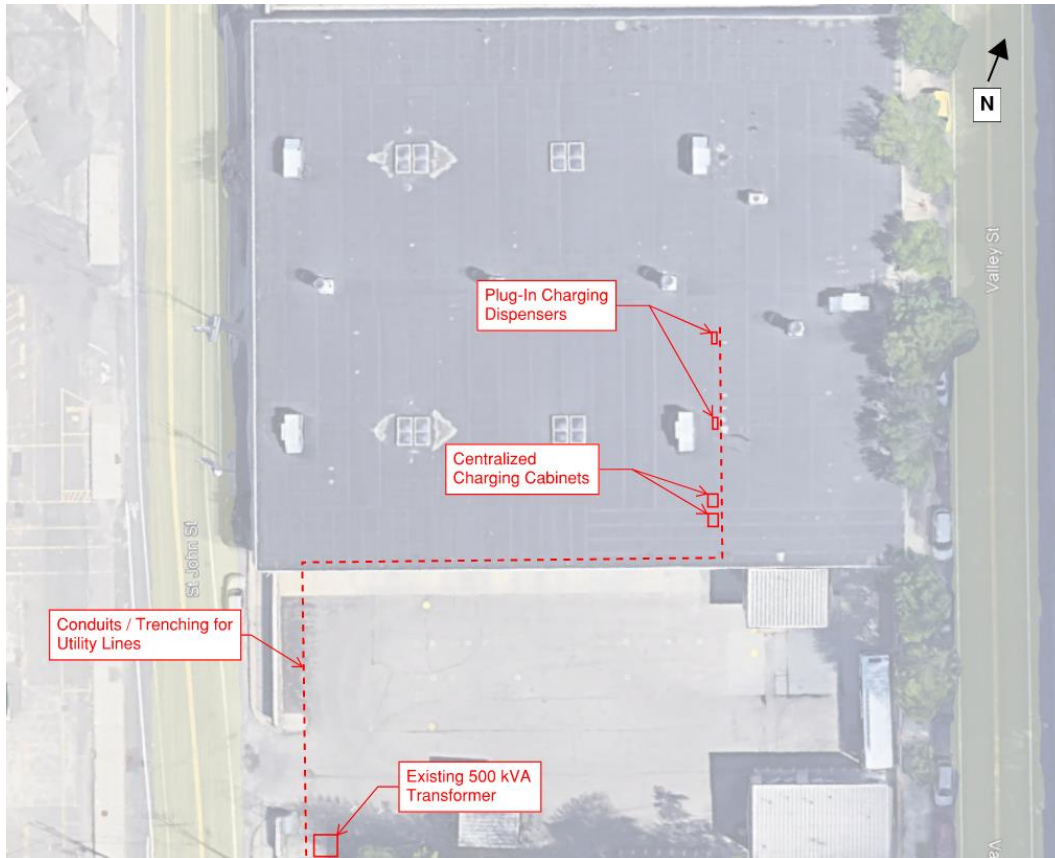
Figure 10 Existing Charging Infrastructure at 114 Valley St
